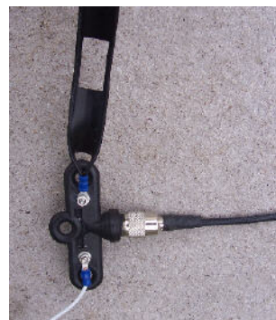
A Typical G7FEK antenna feed point before weatherproofing with self amalgamating tape
