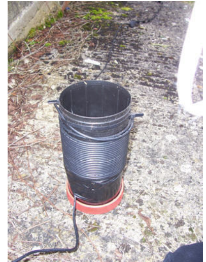
RF Feed line Choke used by G7FEK.
